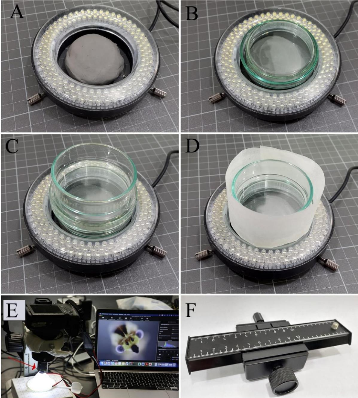
Figure 10. Variations related to the specimens' size or preservation method. A-D) Preparation of the Petri dishes photographing specimens in liquid. Figure D shows the use of the deflector ring in this configuration. E) The microscope objective is jerry-rigged to extension tubes. This system requires smaller domes and lights (as in Figure 3Ae). F) Rail moved using a crank. Photos: C. Flórez-V (E) and J. Cardona-Duque (A-D, F).
